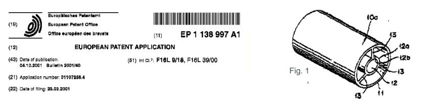
As shown in Fig. 1, a duplex pipe 10 to be used as a work is formed in such a manner that an outer pipe 11, an inner pipe 12 and connecting ribs 13 for connecting together the outer and inner pipes 11 and 12 are moulded of aluminium material by extrusion working or by drawing working into an integrated body. Preferably, the duplex pipe 10 is used as a refrigerant pipe in the cooling cycle of an air conditioner for a car.
