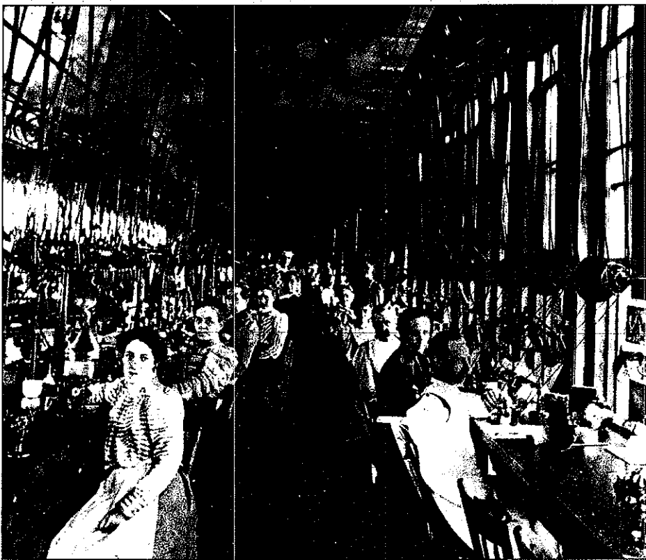
Rows of men and women work with belt-powered machine tools in the screw room at the Elgin National Watch Company, in Elgin, Illinois, May 1899.
