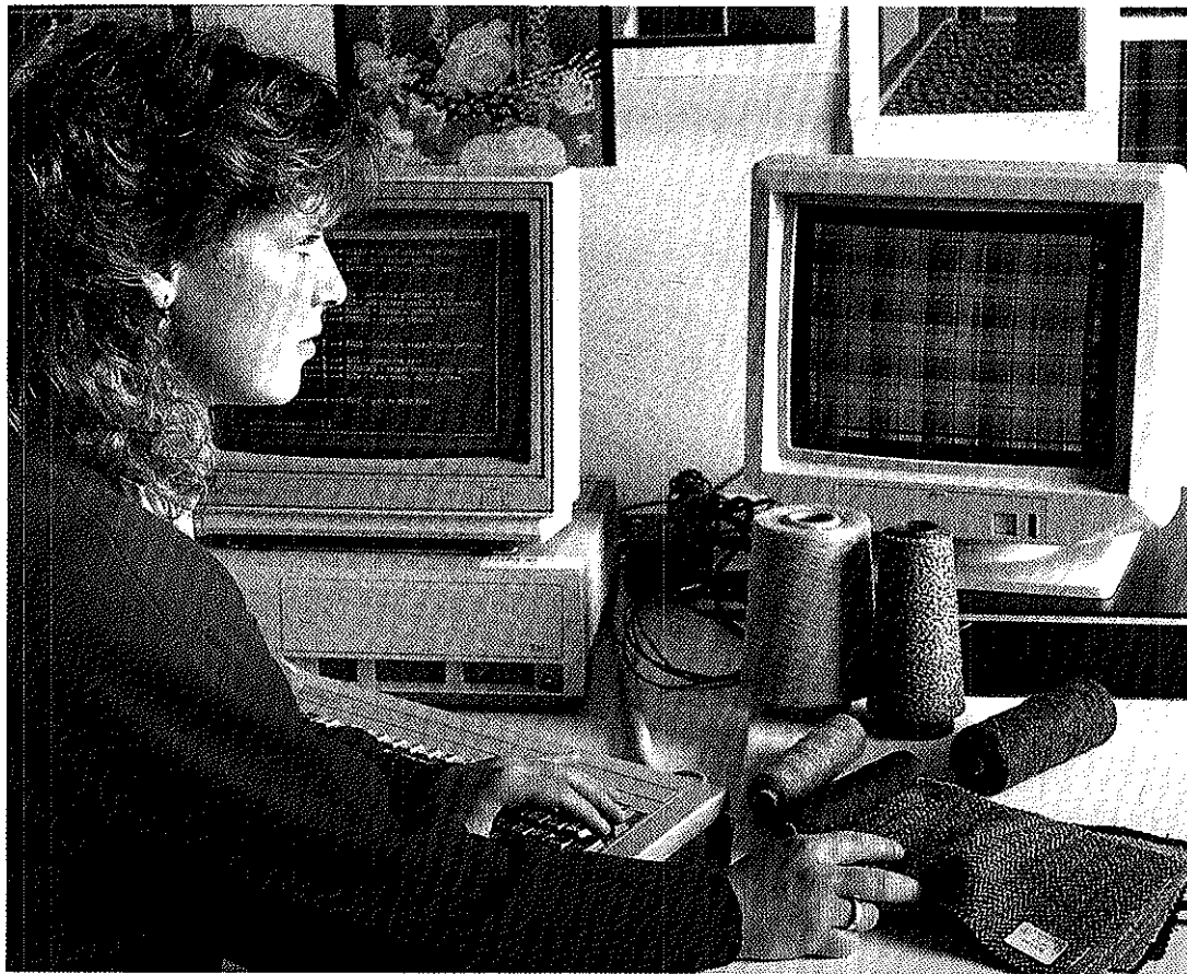
Software developed by the Scottish College of Textiles enables woven fabrics to be simulated on a high-resolution colour monitor using a palette of 16 million colours.
