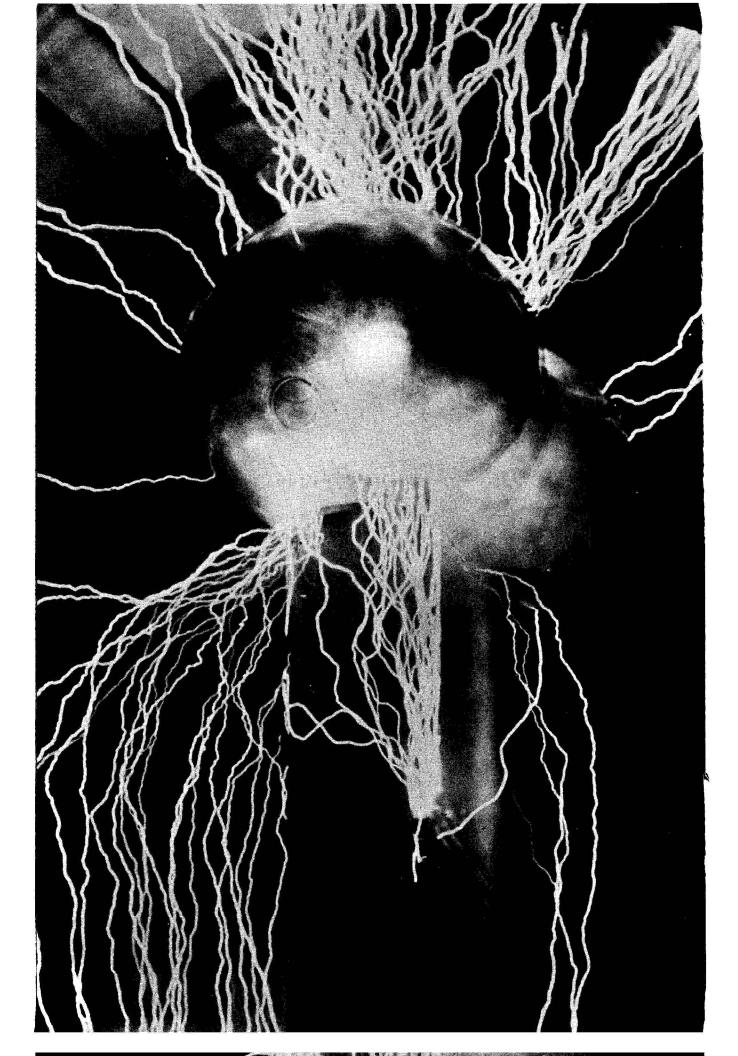
Spectacular arcs of highvoltage electricity crackle around the terminals of the first large Van de Graaff generator in an initial demonstration in 1933. Constructed in a blimp hangar at Round Hill, Mass., it provided an early tool for nuclear research. The project was aided by Research Corporation grants to MIT beginning in 1931.
