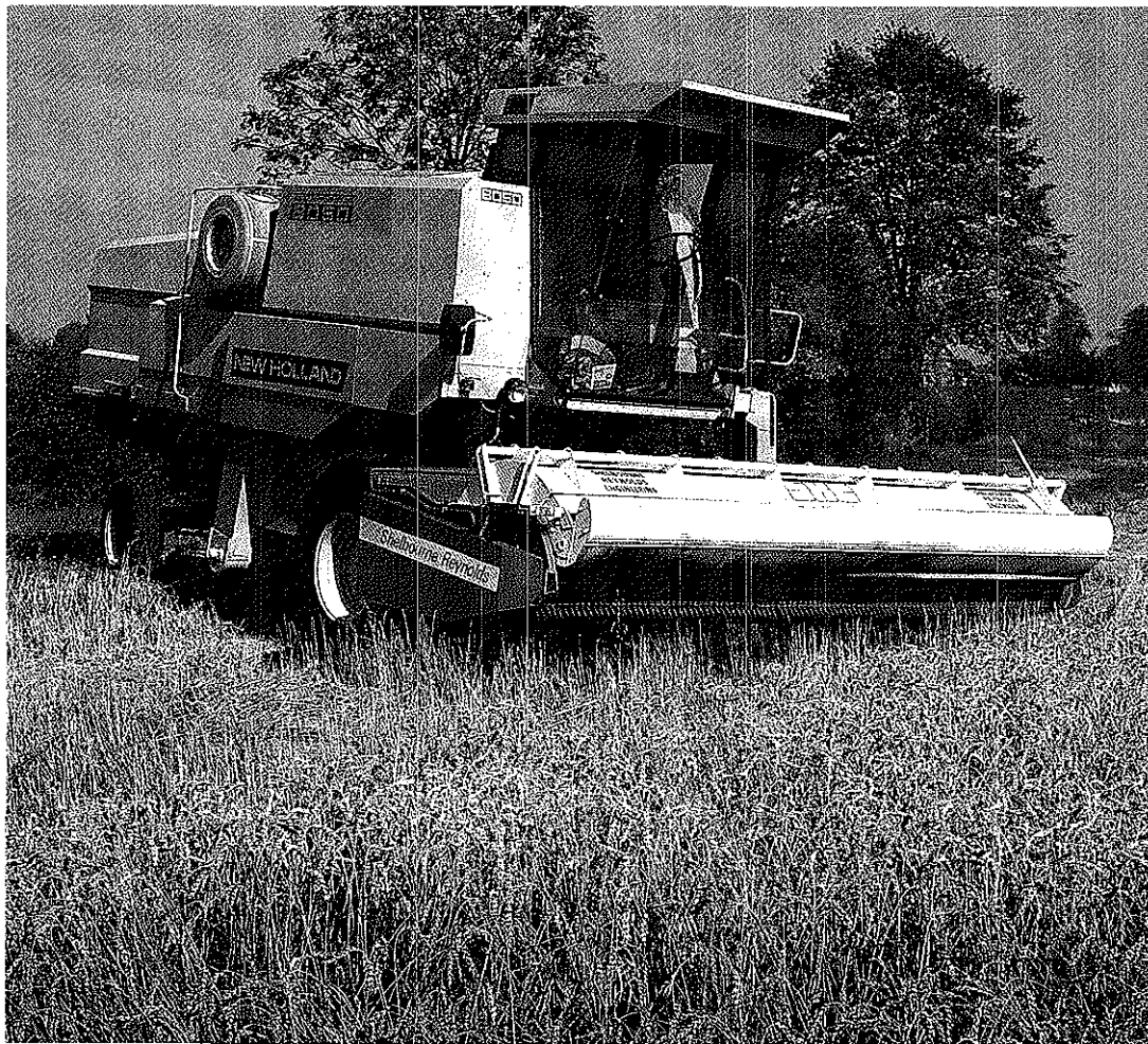
Retrofit grain-stripping header launched by Shelbourne Reynolds under BTG licence at the 1987 Smithfield Show
