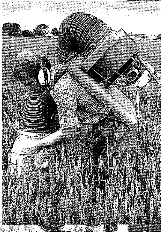
Suction net used to gather fauna from leaves of wheat during Fastac trials. Photo: Shell
