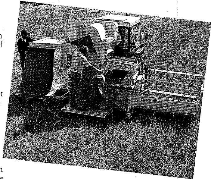
The AFRC Engineering wholecrop harvester collects both grain and straw.
