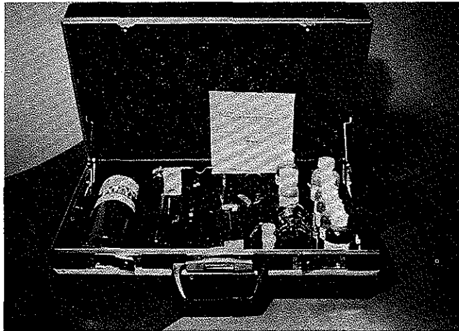
The Civil Engineering Laboratory, Port Hueneme, California developed this compact Kit for identification of weathered paints by field personnel. The Kit is now commercially available.
