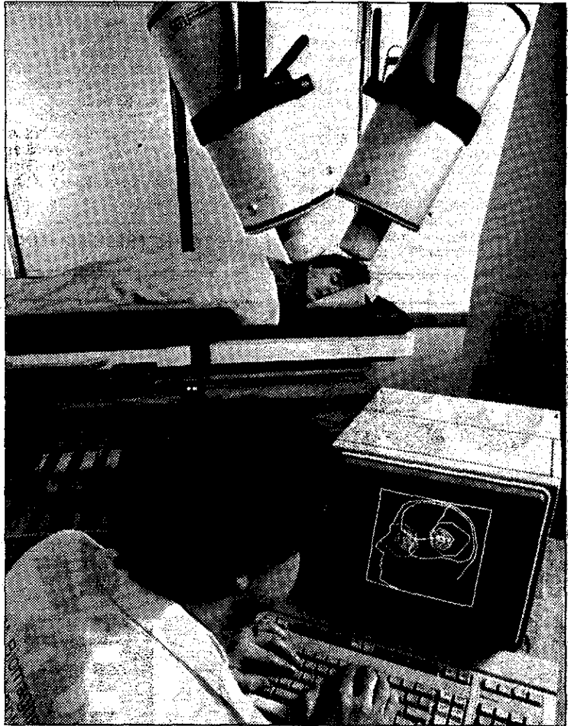
A neuromagnetometer monitors a patient's brain activity. The device, built by Biomagnetic Technologies, uses superconducting materials.
