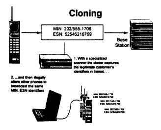
To obtain the ESN/MIN numbers the cloner will typically operate an electronic scanning device near a busy highway, tunnel. or airport -- anywhere there is likely to be a high density of traffic transmitting ESN/MIN pairs to the wireless system. Once the scanner has captured an ESN/MIN pair, the cloner reprograms the stolen ESN/MIN pair into other phones so they will mimic the legitimate customer's handset. Programming a
