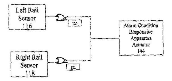
(*Safe Bed's Reply*, at 27). While Safe Bed's diagram is not clear on this point, the idea is to simplify the dual structure of OR-gates 120 and 122 by replacing them with a single equivalent OR-gate 120/122. (*Safe Bed's Reply*, at 27). According to Safe Bed:
