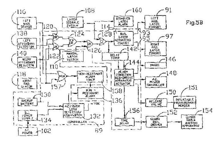
This diagram covers quite a bit that is not germane to claim 50. The pertinent signal or signals in this instance originate at the left rail sensor 116 and/or the right rail sensor 118. In order to actuate the adjustment prevention means, the signal must make its way to the responsive apparatus actuator 144. As a result, the parties agree that the diagram may be redacted to depict the elements at issue here, up to a point:
